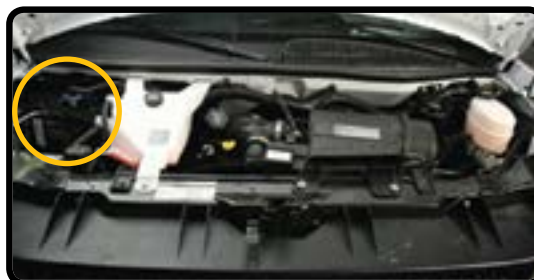
Disconnect the 12V Battery Cables
