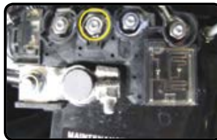
Main Fuse Box Power Supply Cable
