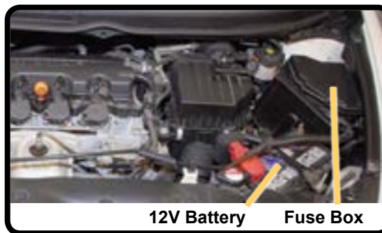
Fuse Box and 12V Battery Location
