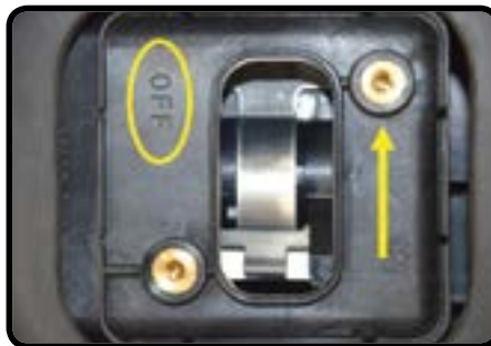
HV System Disconnect Switch
