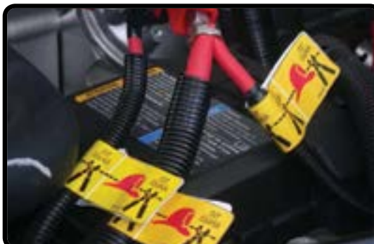
Cut 3 Exposed Cables (Alternate Procedure)
