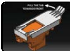
HV Service Disconnect Detail
