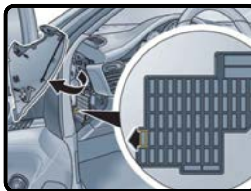
Fuse Box - Fuse 46 Location
