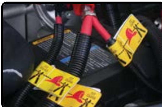
Cut 3 Exposed Cables (Alternate Procedure)
