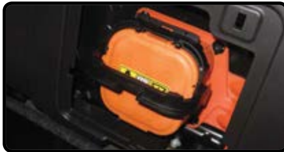
Remove Upper Service Disconnect Fully
