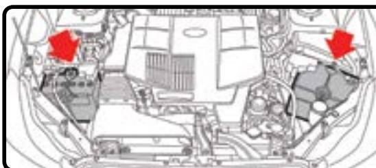
12V Restart and Auxiliary Battery
