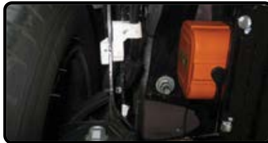
Remove Lower Service Disconnect Fully
