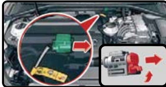
Disconnect HV Emergency Disconnect
