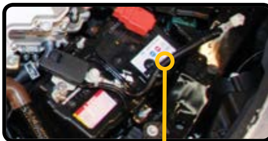
Cut Negative 12V Battery Cable
