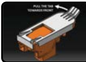
HV Service Disconnect Detail
