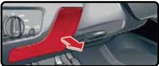
Fuse Box Left of Steering Column
