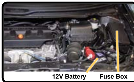
Fuse Box and 12V Battery Location
