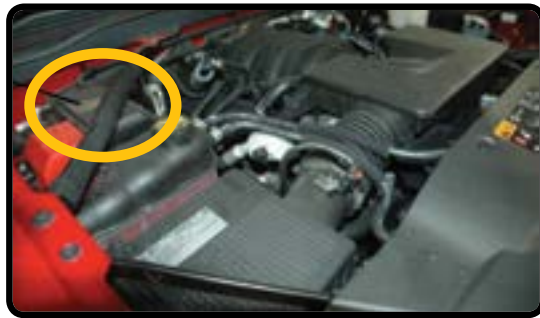
Disconnect 12V Negative Battery Cable
