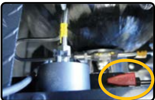
Turn Isolation Valve Counter Clockwise
