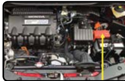
Positive Battery Terminal
