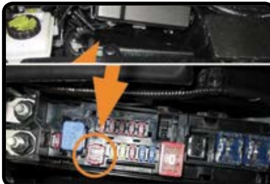
Fuse and Box in Engine Compartment
