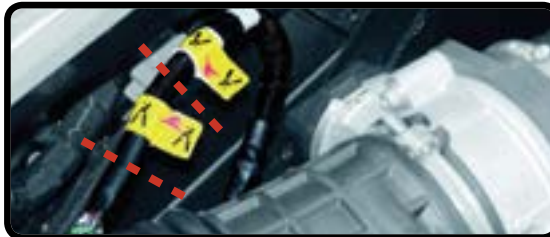
Cut 12V Battery Negative Cable As Marked
