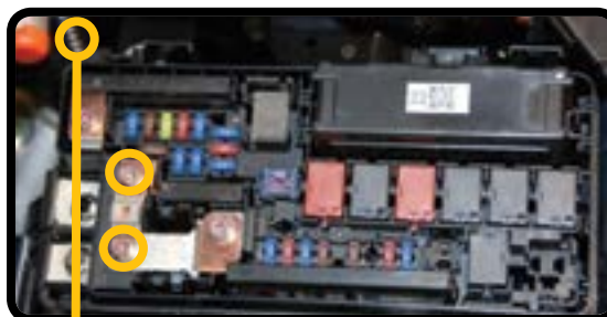
Cut Cable and Main Fuse Screw Locations
