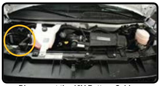
Disconnect the 12V Battery Cables
