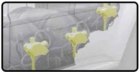
Pressure Relief Valve - Drivers Side View
