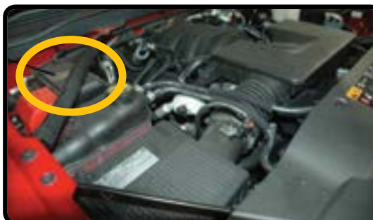
Disconnect 12V Negative Battery Cable
