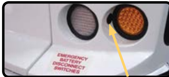
Curb-side Rear Fender Access Push-Button
