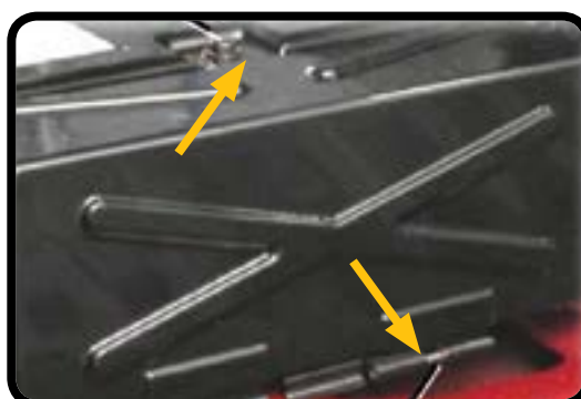
A 10 mm hex bolt secures the module. Hinges are attached to the battery cover.
