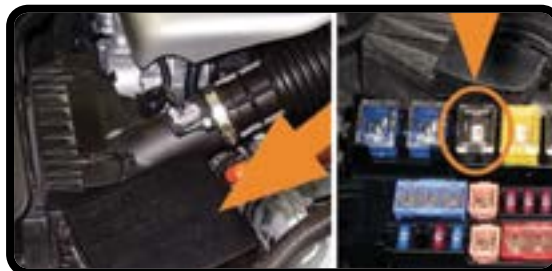
Fuse and Box in Engine Compartment
