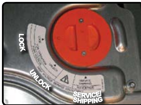
High-Voltage Service Disconnect Switch Shown in LOCK position
