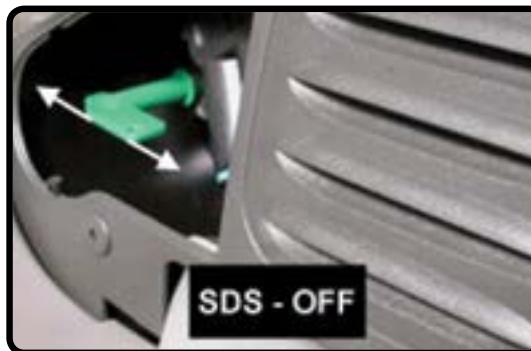
Service Disconnect Switch
