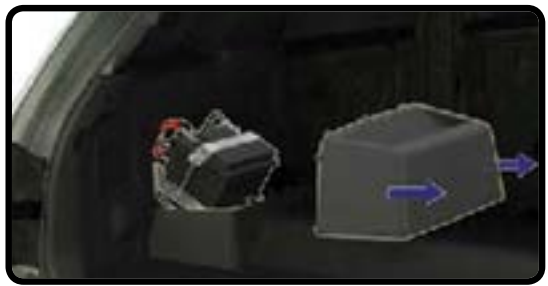
Disconnect the 12V Negative Cables
