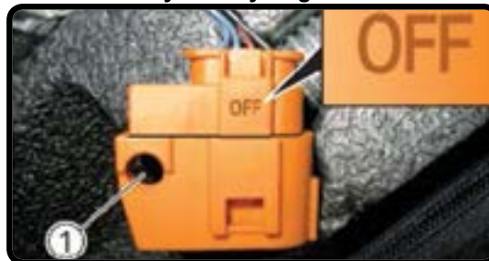
High Voltage Safety Connector
