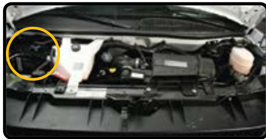
Disconnect the 12V Battery Cables
