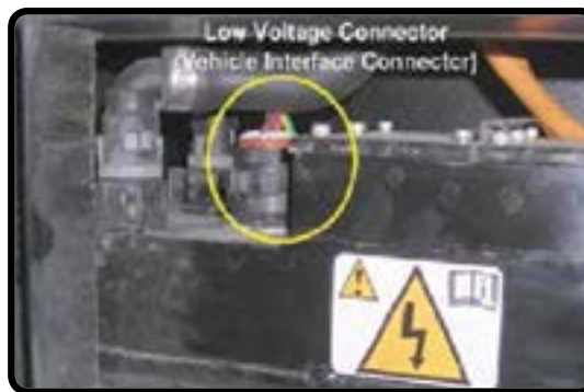
Disconnect the Low Voltage Connector Underneath the Front Edge of HV Battery
