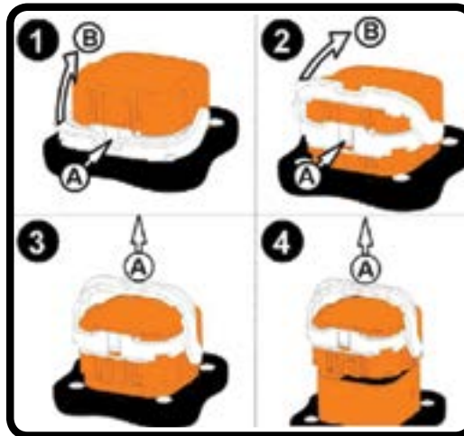
Manual High Voltage Disconnect Located Under Rear Seat Cushion
