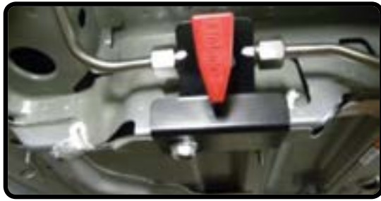
1/4 Turn Shut-Off Valve, Off Points Down
