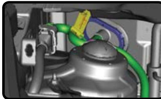
12V Wire Harness Behind Tower Strut, Engine Compartment, Passenger's Side
