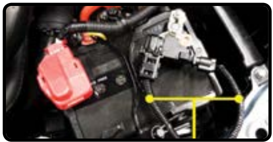
Cut the Negative Cables
