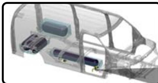
Isolation Valve Location
