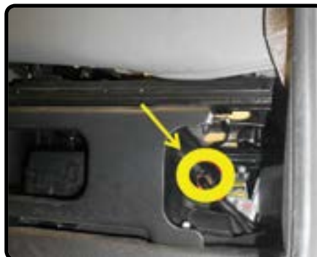
HV Disconnect Under Driver's Seat
