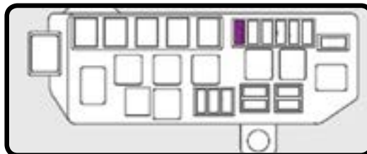
Fuse No. 7 Location
