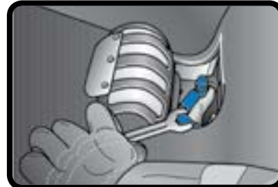
Disconnect the Ground at the Threaded Connection
