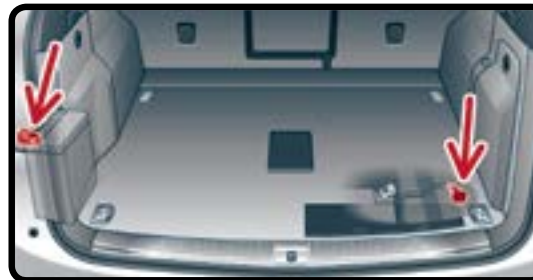
Disconnect the Ground Cables
