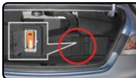
Service Disconnect Located in Trunk
