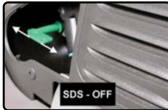
Service Disconnect Switch
