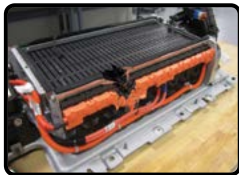
Damaged High Voltage Battery
